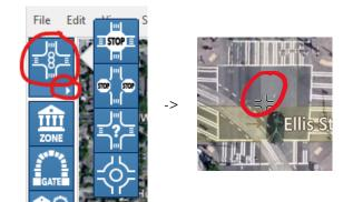
*Right-Click:* A signalized intersection can be placed at the mouse position by using the *Right-Click* button on a roadway segment's Leg or on at a location on the base map. The right-click will open the context menu. Then select **Insert Intersection -> Signalized**.
